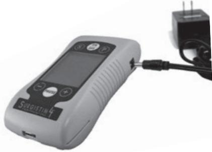
Press the (PAUSE) button to pause stimulation before connecting or disconnecting the AC Adapter. Press (PAUSE) to resume treatment.
